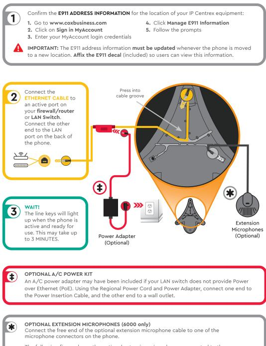
The following figure shows the optional extension microphones connected to the microphone connectors on the phone.
