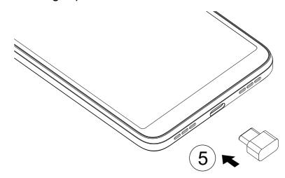
It is advised that you fully charge your battery before first use ( \( \subseteq \)]. Connect the charger to your phone and an outlet. Charging status is indicated by the percentage on screen while the phone is powered off. The percentage increases as the phone is charged.
